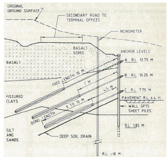
*Geotechnical aspects of the Anchored Sheet Pile Retaining Wall constructed in 1982*
