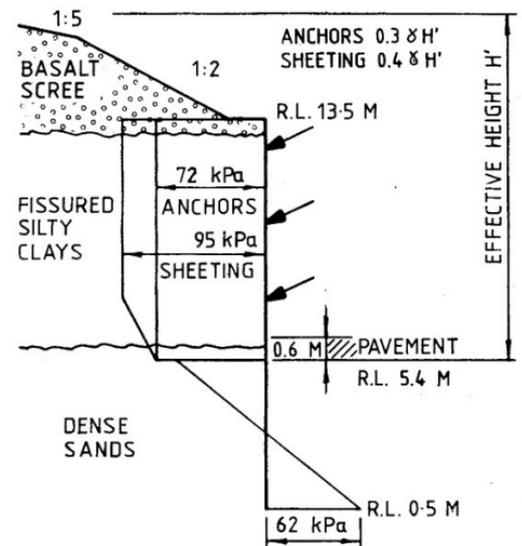
*Earth pressure diagram for 3 level anchored wall*
