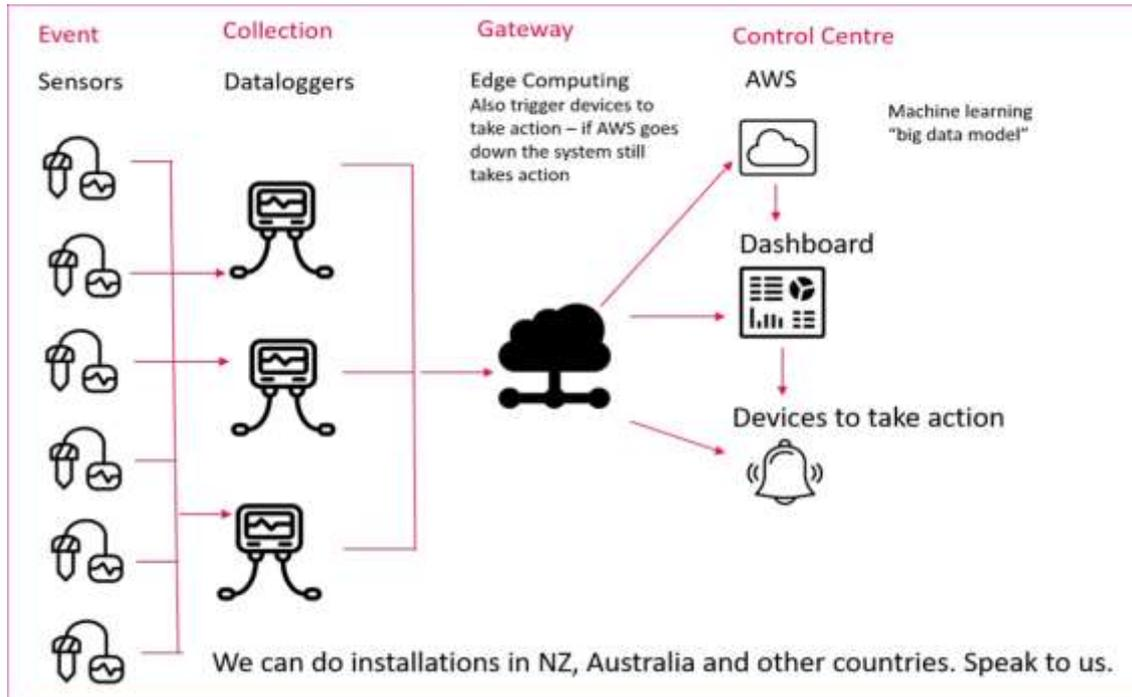
Data are stored within the station and also streamed to the cloud using either mobile phone/data (low-power CatM1), LoRa or satellite networks. Viotel's cloud platform has been built in partnership with Amazon Web Services, using high security certificate exchange to validate connections and encrypted data flows.
